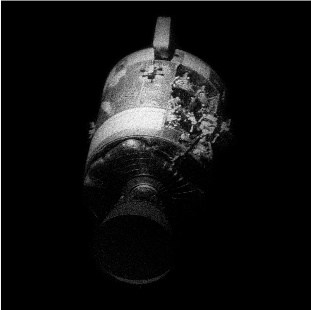
View of the severely damaged Apollo 13 Service Module after separation, 17 April 1970. (Image: NASA)
