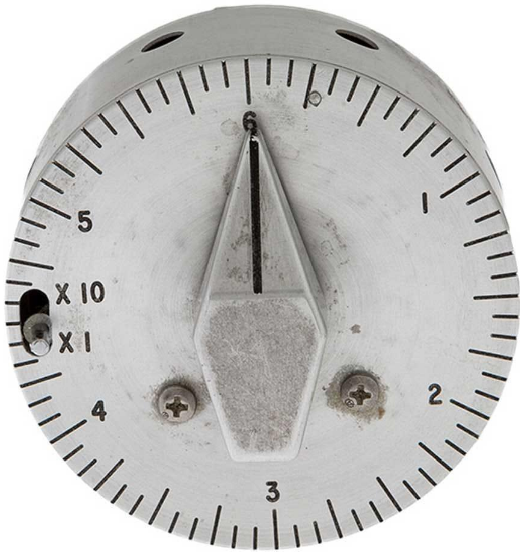
Command Module Interval Timer from Apollo 12, in stainless steel
