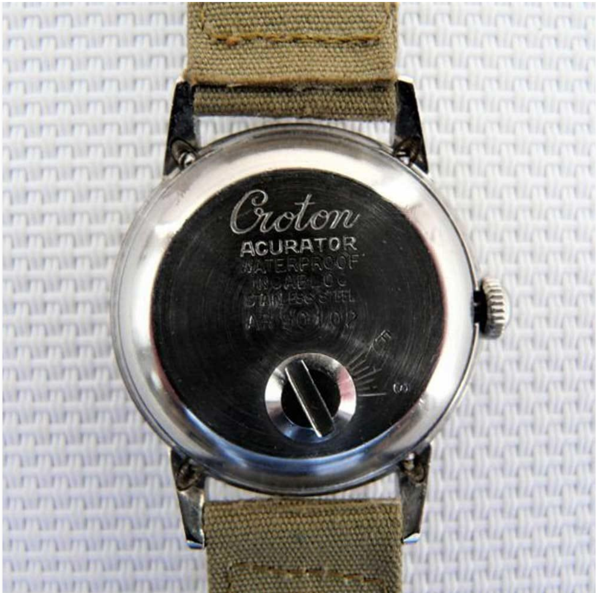
A screw on the Croton Acurator's caseback allowed rate adjustment without opening up the watch. (Image: Catawiki)
